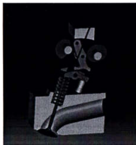
Fig. 1. Helical torsion spring in valve timing mechanism
